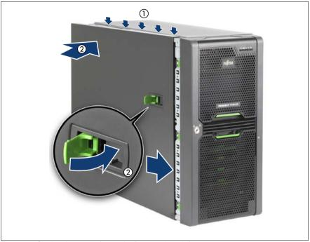
Figure 38: Closing the server (example: floorstand model)
